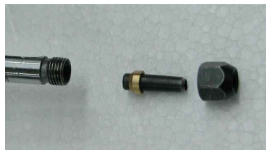
4 After releasing bolt, now you can replace punch blade with as you want. Please watch out the direction of "CORK".
